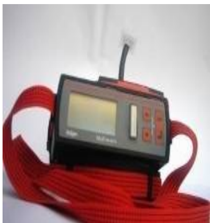
Plate (3-11), View of Gas analyser Drager- Multiwarn/ Germany
